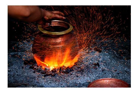
Copper is one of the best metals for conducting heat and was often used in cooking vessels, so that the heat spread evenly across the surface of the pot. The metal can, however, react with acidic foods to produce toxins, so in workshops like these the pots are lined with tin on the inside. This profession is now vanishing due to the availability of cheaper stainless steel vessels.
